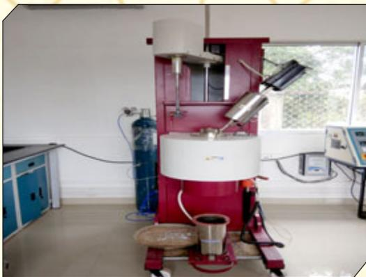
Stir Casting Furnace (9000C)
